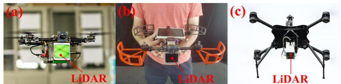
Fig. 6. Three different platforms: (a) 280  $mm$  wheelbase small scale quadrotor UAV carrying a forward-looking Livox Avia LiDAR, (b) handheld platforms, (c) 750  $mm$  wheelbase quadrotor UAV carrying a down-facing Livox Avia LiDAR. All three platforms carry the same DJI Manifold-2C onboard computer. The video of real-world experiments is available at <https://youtu.be/20vjGnxzf8>.
